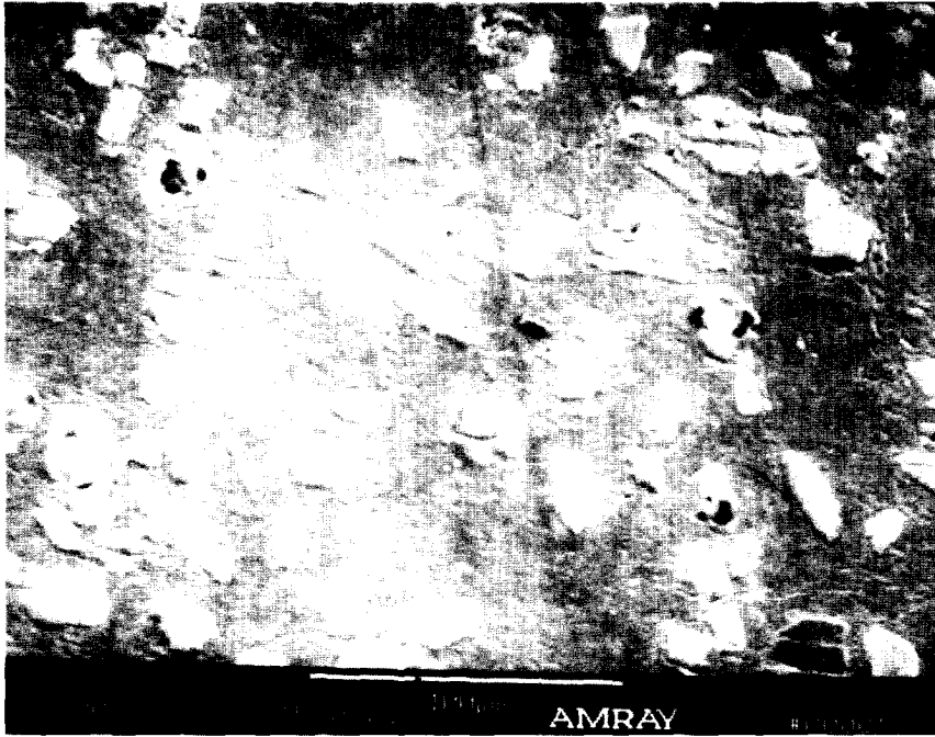
Fig. 13. Micrograph of the fractured composite taken along the tensile axis showing the development of cracking within the particles.
